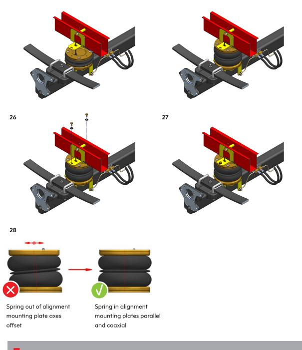
**CAUTION!** - Before fully tightening the bolts that secure the air spring to the upper and lower brackets, set the vehicle at ride height (spring height approximately 13..14 cm) and ensure that the springs are correctly aligned.
